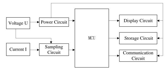
Figure 1 the overall principle block-diagram
